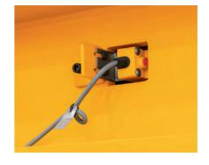
Blade Breakage Detector If any blade breakage occurs during cutting, the machine will automatically stop to ensure safety of operator and machine.
